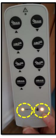
To unlock the remote control, use the black magnet attached to the lead and swipe it over the unlock symbol on the bottom right part of the remote control – the light will come on
